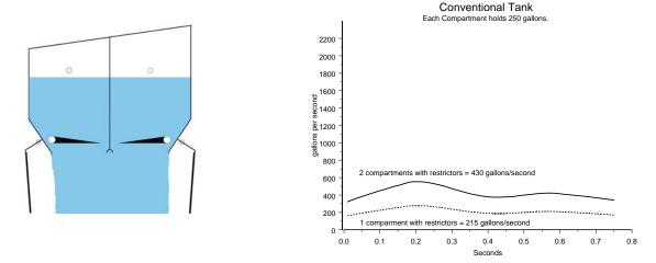
The figure to the left above shows two compartments released simultaneously with restrictors down. Each compartment flows at about an average of 215 gallons per second. The dotted line shows the flow rate for one compartment while the solid line shows the flow rate for two.
