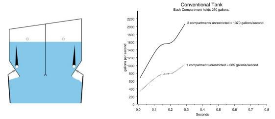
The figures above illustrate the same thing but without the restrictors deployed. Each compartment flows about an average of 685 gallons per second.
