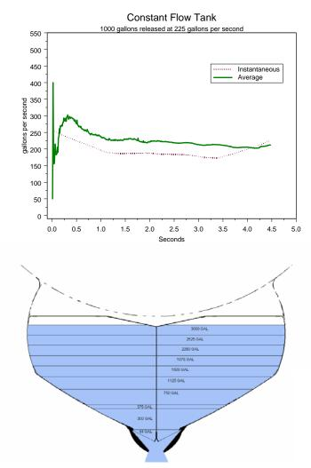
Constant flow systems have door controls that allow the delivery system to behave as a single tank. Once the drop controller establishes the flow rate, the coverage level produced remains constant over the duration of the drop. The effect of changing the volume released will only change the length of the drop, not the flow rate.
