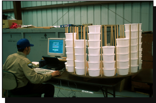
Figure 8—The weigher removes sorted cups from the carousel and places them on a balance. A computer records the weight of each cup.
