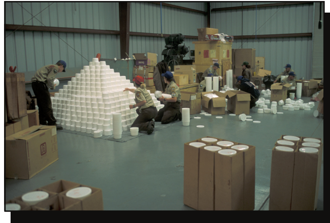
Figure 9—Cups from water or foam drops can be stacked pyramid style to dry before being used again.
