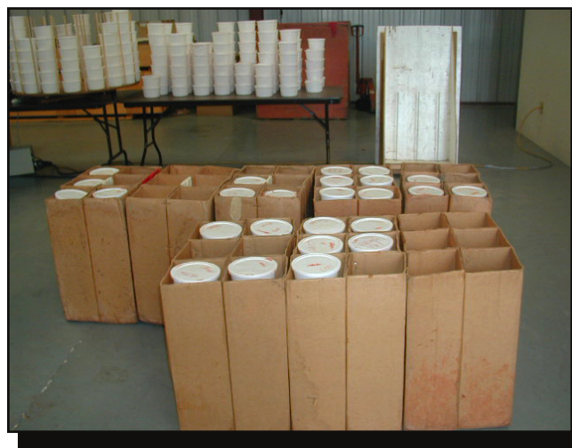
Figure 7—Pickup boxes (foreground), disgorging apparatus (right rear), presorted cups (center table), and sorted cups on carousel (left rear).
