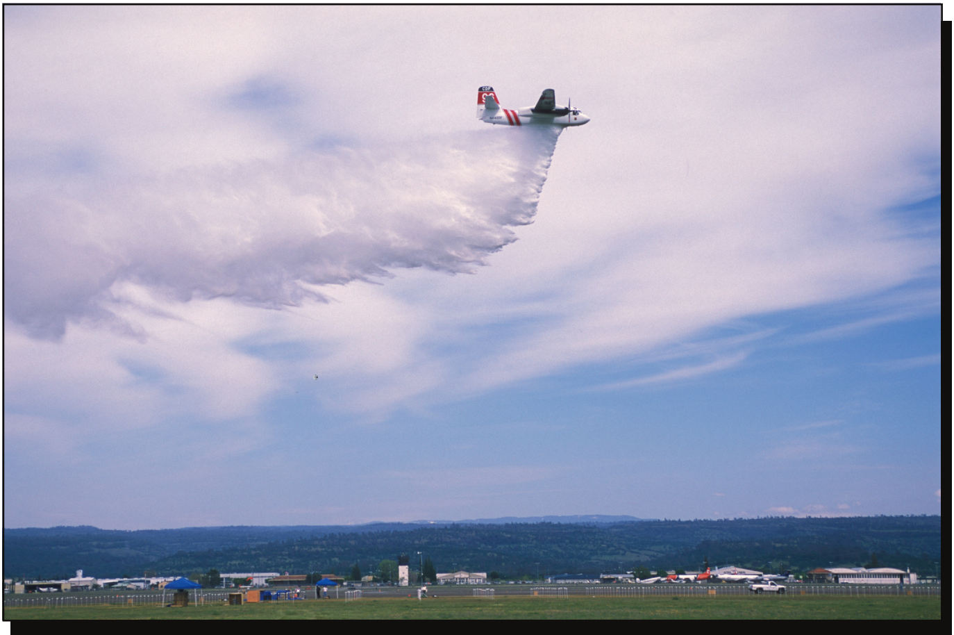
Figure 1—Airtanker dropping water over a grid of cups during a drop test.
