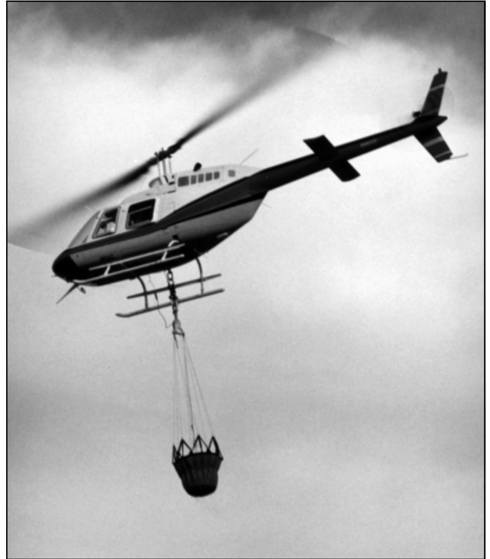
Figure 8—Drop test of the Forest Service Bell 206 with 100-gallon Bambi helibucket.
