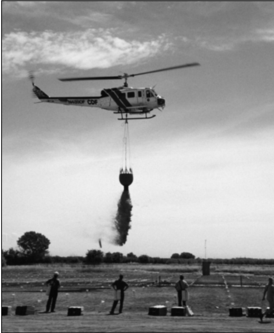
Figure 8—Drop test of the CDF Bell S205 with 240-gallon Bambi helibucket using gum-thickened retardant.
