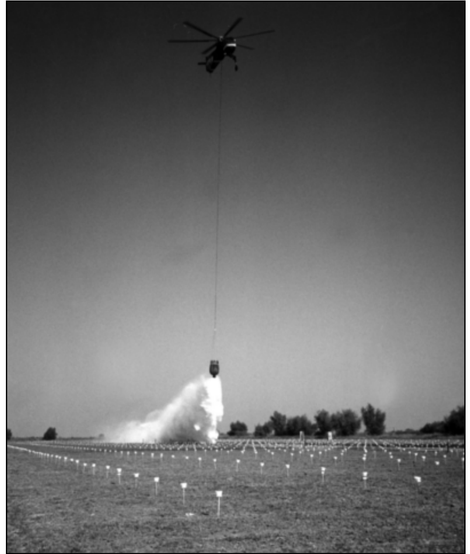
Figure 8—Drop test of the Siller Brothers S-64 with 2,000-gallon Bambi helibucket.
