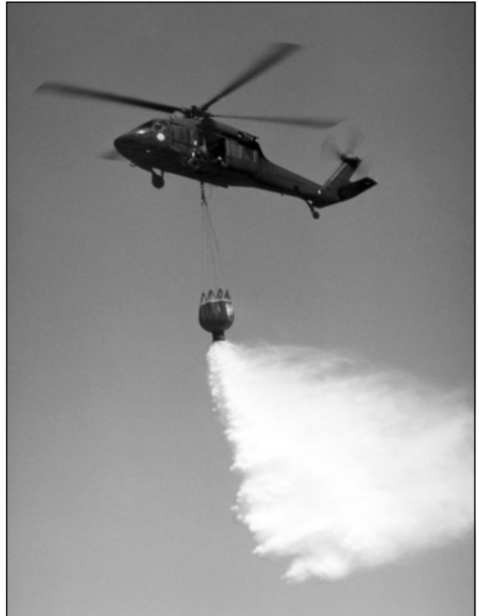
Figure 14—Drop test of the National Guard Black Hawk with 660-gallon Bambi helibucket using water.
