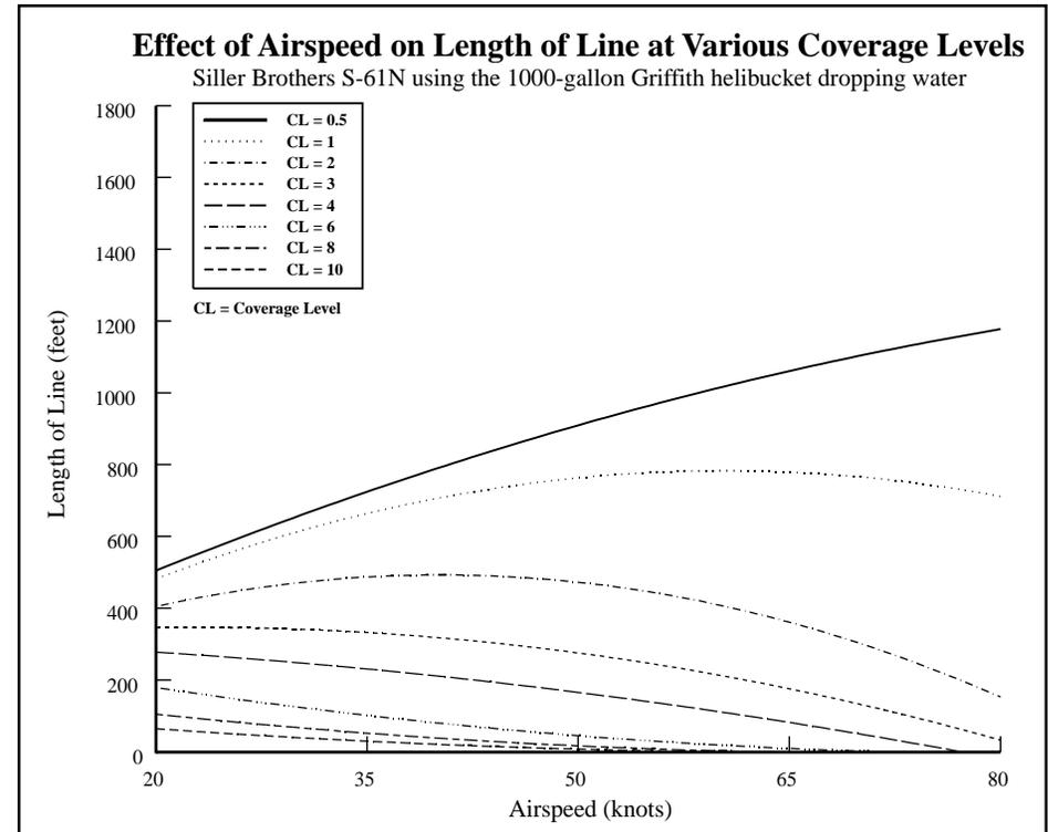
Figure 6—Use this graph to estimate the drop speed needed to produce the maximum line length of water at various coverage levels.
