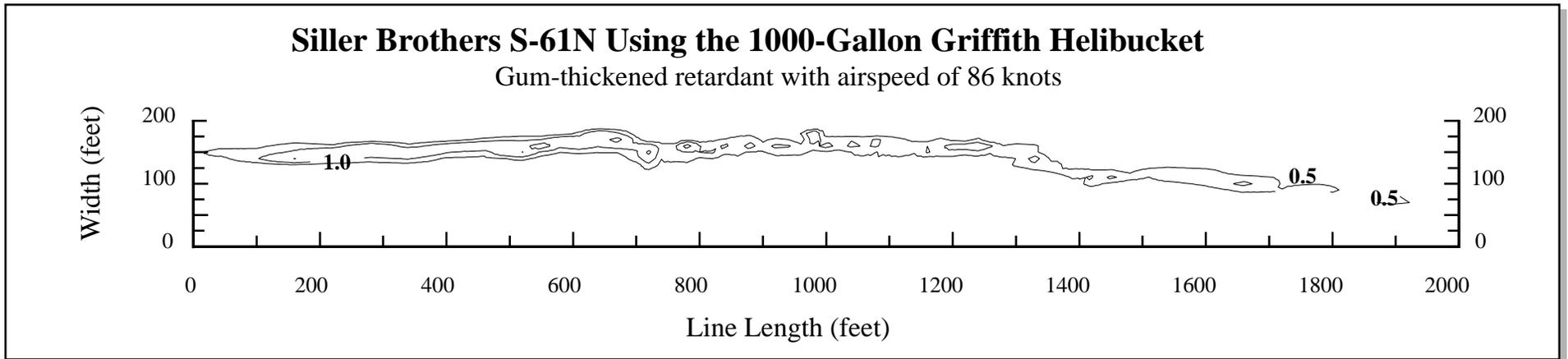
Figure 5—Drop pattern characteristics for the Siller Brothers S-61N helicopter using the 1000-gallon Griffith helibucket with gum-thickened retardant at an airspeed of 86 knots (99 mph) and a drop height of 85 feet. The contour lines are at coverage levels of 0.5, 1, 2, 3, 4, 6, 8, and 10 gallons per 100 square feet.
