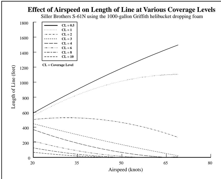
Figure 7—Use this graph to estimate the drop speed needed to produce the maximum line length of foam at various coverage levels.
