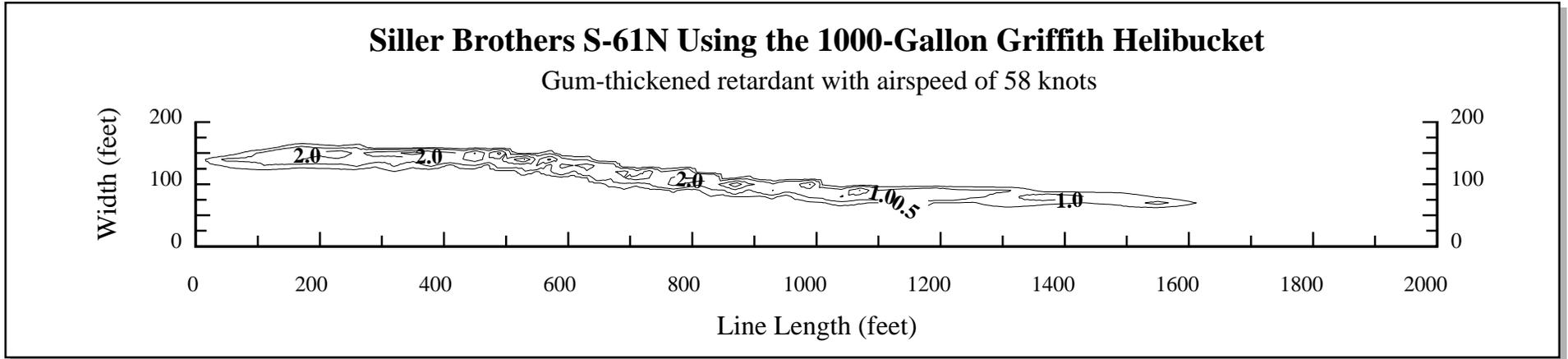
Figure 4—Drop pattern characteristics for the Siller Brothers S-61N helicopter using the 1000-gallon Griffith helibucket with gum-thickened retardant at an airspeed of 58 knots (67 mph) and a drop height of 60 feet. The contour lines are at coverage levels of 0.5, 1, 2, 3, 4, 6, 8, and 10 gallons per 100 square feet.
