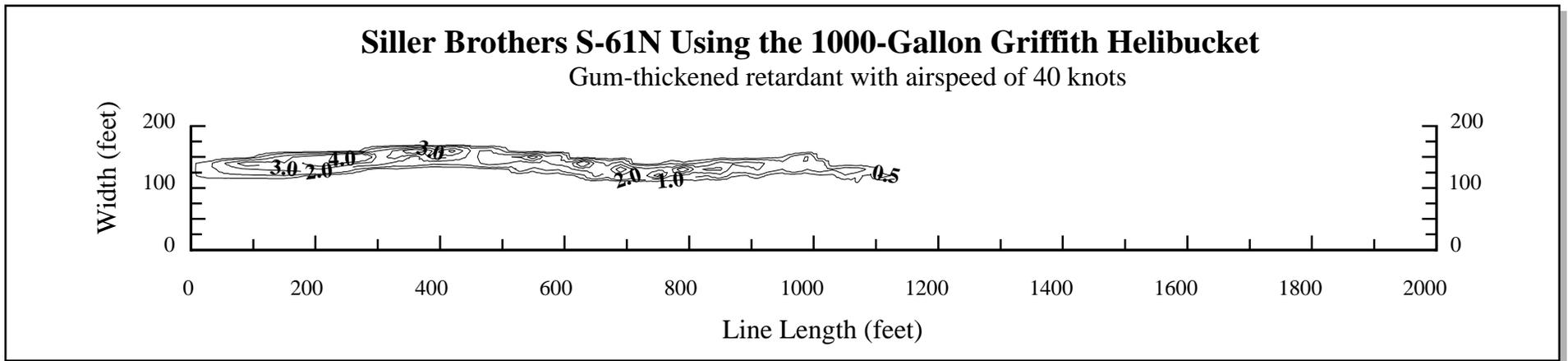
Figure 3—Drop pattern characteristics for Siller Brothers S-61N helicopter using the 1000-gallon Griffith helibucket with gum-thickened retardant at an airspeed of 40 knots (46 mph) and a drop height of 76 feet. The contour lines are at coverage levels of 0.5, 1, 2, 3, 4, 6, 8, and 10 gallons per 100 square feet.
