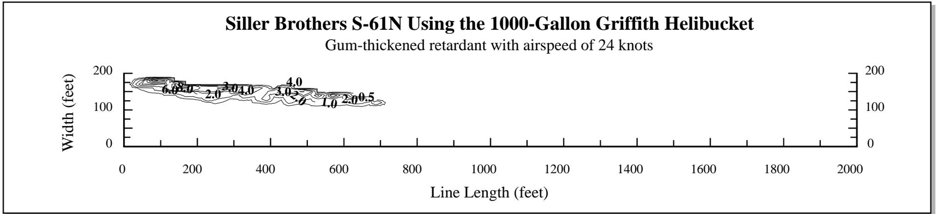
Figure 2—Drop pattern characteristics for the Siller Brothers S-61N helicopter using the 1000-gallon Griffith helibucket with gum-thickened retardant at an airspeed of 24 knots (28 mph) and a drop height of 60 feet. The contour lines are at coverage levels of 0.5, 1, 2, 3, 4, 6, 8, and 10 gallons per 100 square feet.
