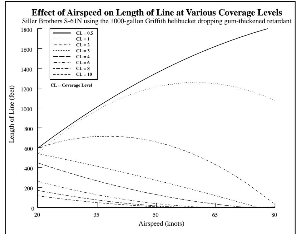
Figure 8—Use this graph to estimate the drop speed needed to produce the maximum line length of gum-thickened retardant at various coverage levels.
