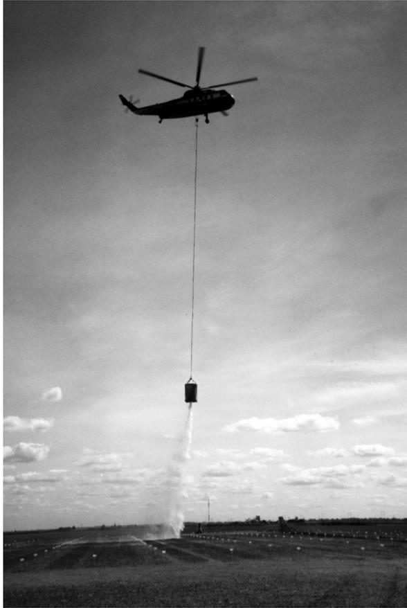
Figure 9—Drop test of the Siller Brothers S-61N helicopter using the 1000-gallon Griffith helibucket dropping water.
