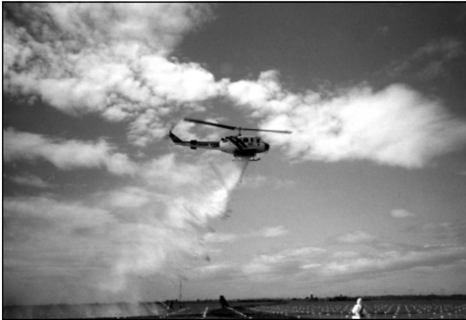
Figure 7—Drop test of the LA County Bell S205 helicopter using the Sheetcraft fixed tank to drop water.
