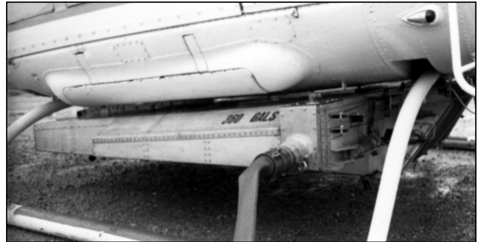
Figure 1—The LA County Bell S205 helicopter with the Sheetcraft fixed tank.
