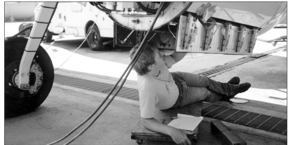
Figure 1 —The constant flow tank for the AeroUnion SP-2H.
