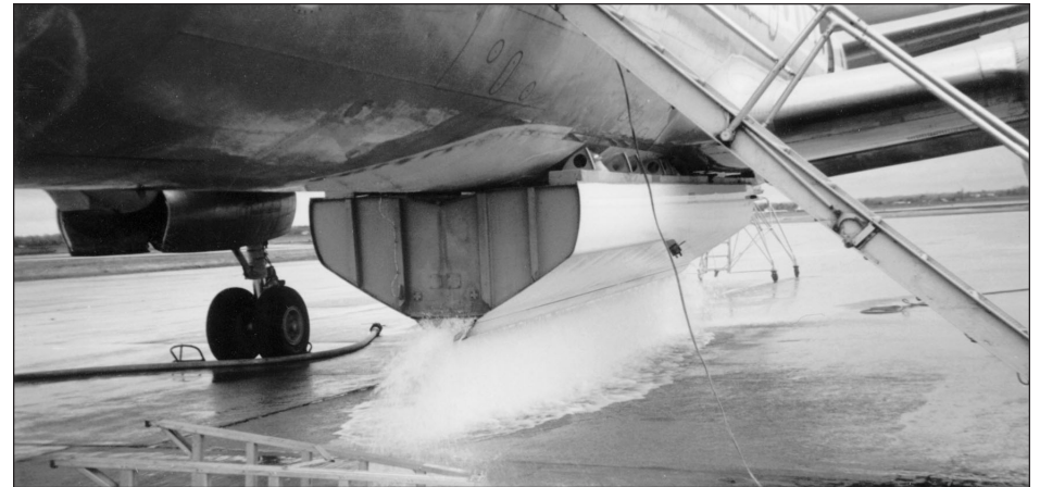
Figure 1 —The Constant flow tank of the Airspray Electra L-188.
