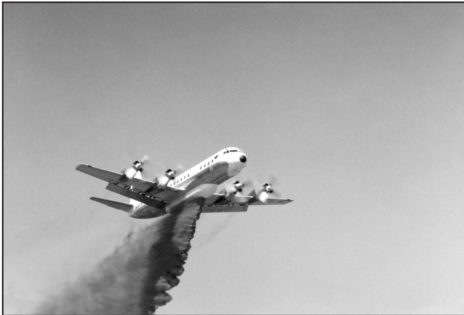
Figure 6—Drop test of the Airspray Electra L-188.
