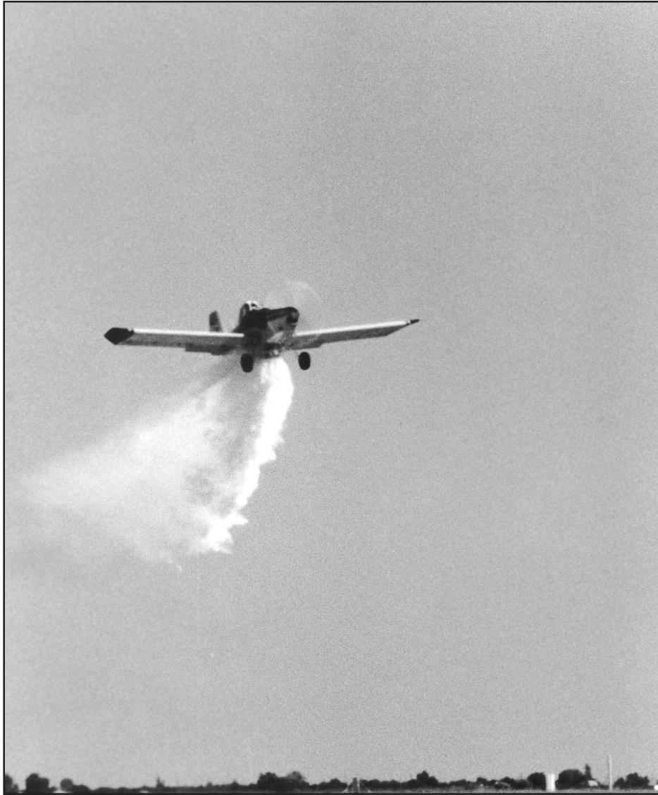
Figure 3—Drop test of the Marsh Turbo Thrush.
