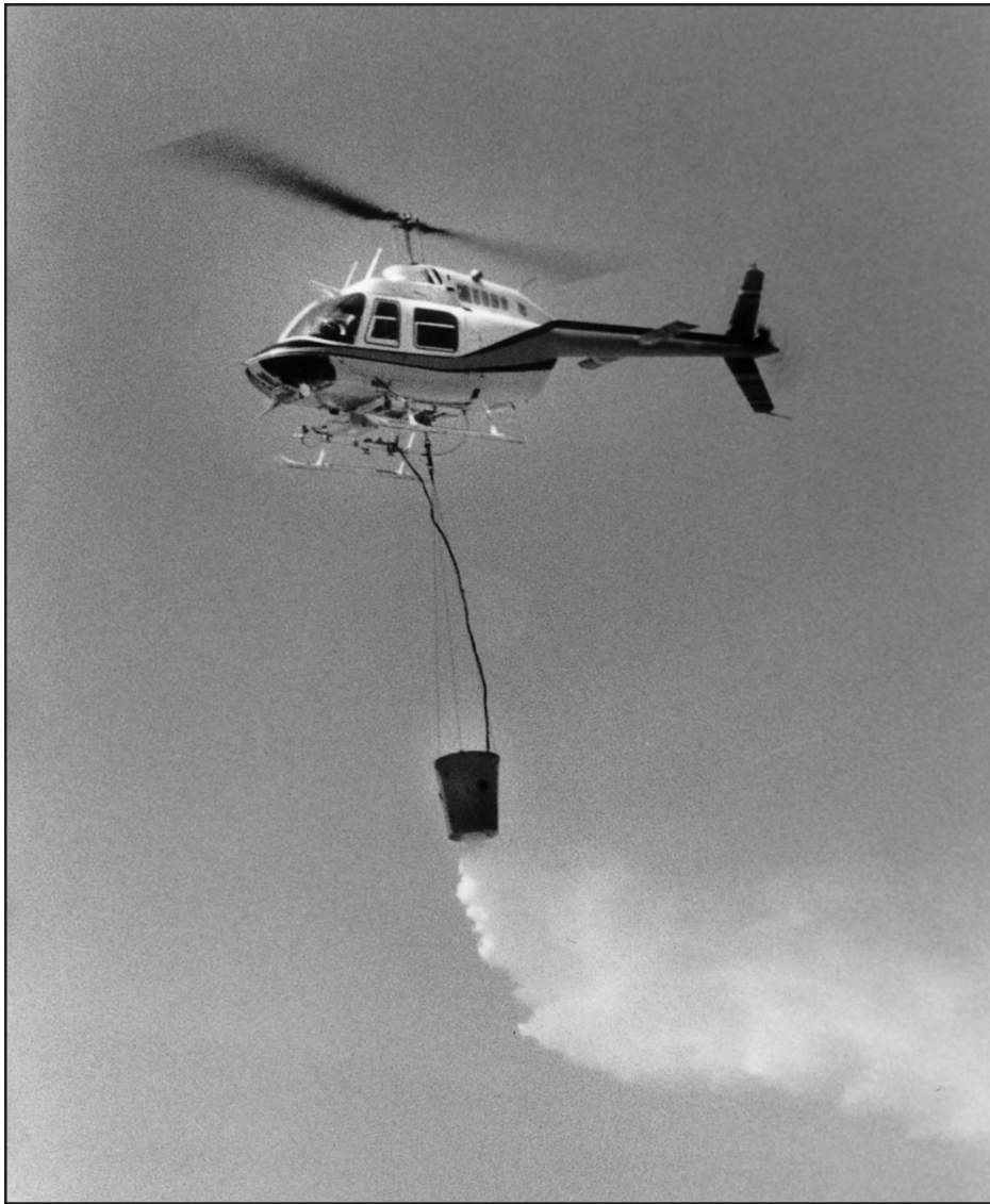
Figure 8—Drop test of the Griffith 100-gallon helibucket.
