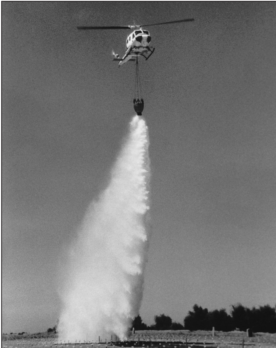
Figure 8— Drop test of the Bambi 324-gallon helibucket.
