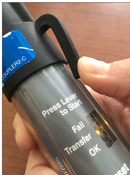
Figure 4.11. Photograph showing Onset HOB0 Waterproof Shuttle with coupler pressed and a lit yellow Transfer light. A flashing Transfer light indicates that data is in the process of being transferred from a data logger to the shuttle.
