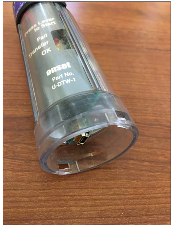
Figure 4.8. Photograph showing Onset HOB0 Waterproof Shuttle with circuit board reinstalled correctly. Note the USB port facing the open end and the LEDs are visible through the opening on the label.
