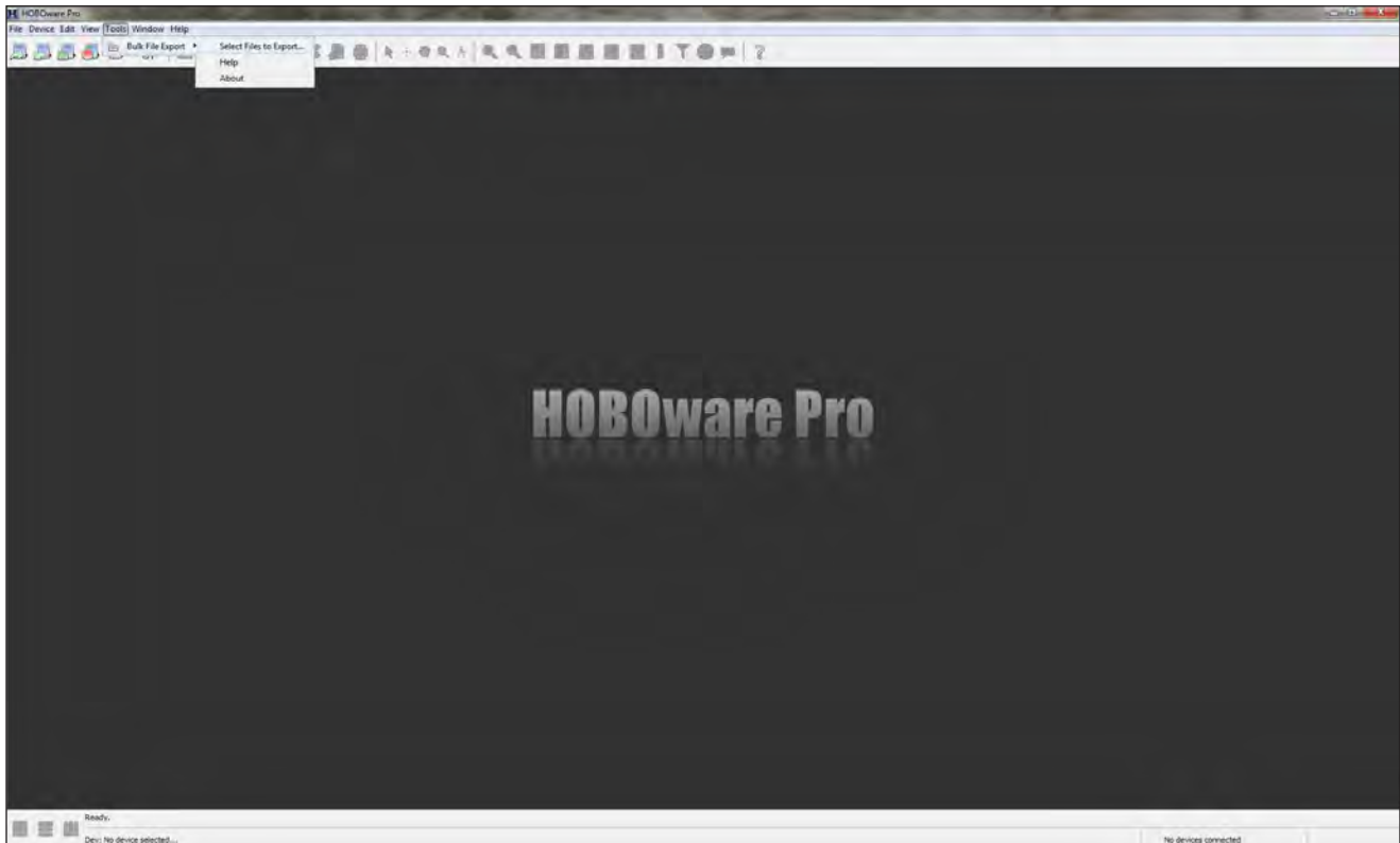
Figure 2.9. Screen capture showing HOBOWare Pro Select Files to Export... option under the Bulk File Export option, under the Tools menu.
