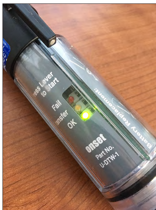
Figure 4.12. Photograph showing Onset HOB0 Waterproof Shuttle with a lit green OK light. A flashing OK light indicates that data transfer process from data logger to shuttle is complete.
