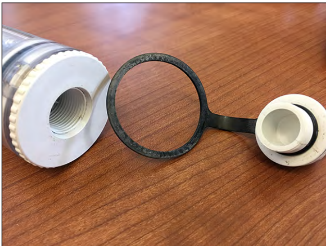
Figure 4.4. Photograph showing Onset HOBOWare Waterproof Shuttle with center cap and rubber loop removed.
