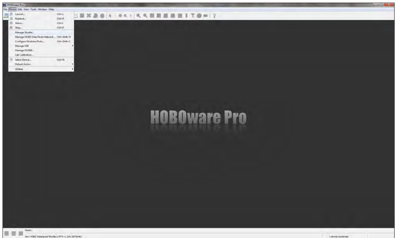
Figure 4.2. Screen capture showing HOBOWare Pro Manage Shuttle... option under the Device menu.
