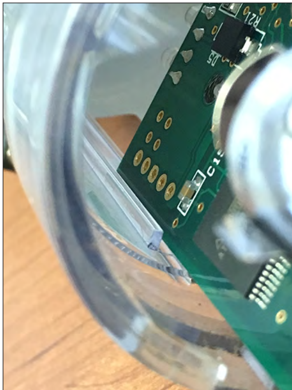
Figure 4.7. Photograph showing close-up of Onset HOB0 Waterproof Shuttle with circuit board aligned with shuttle housing slots.
