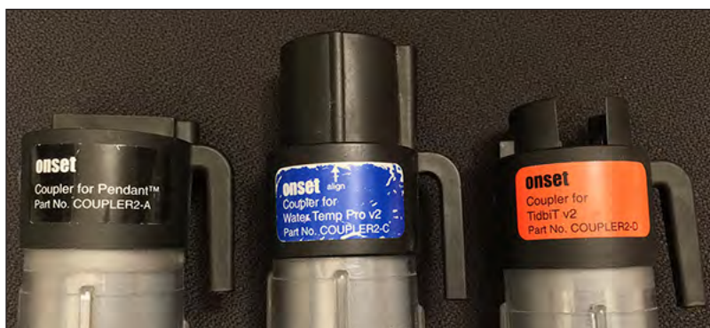
Figure 1.9. Photograph showing Onset couplers for Onset data loggers. From left to right: Coupler2-A for Pendant data loggers, Coupler2-C for U22 data loggers, and Coupler2-D for TidbiT data loggers.
