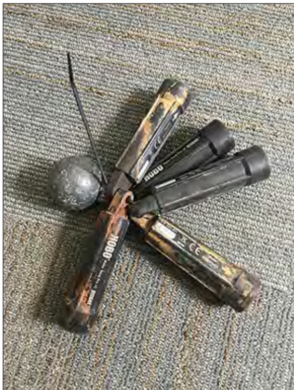
Figure 2.2. Photograph showing five Onset U22 data loggers attached to a 10-ounce lead weight with an 8-inch cable/zip tie.
