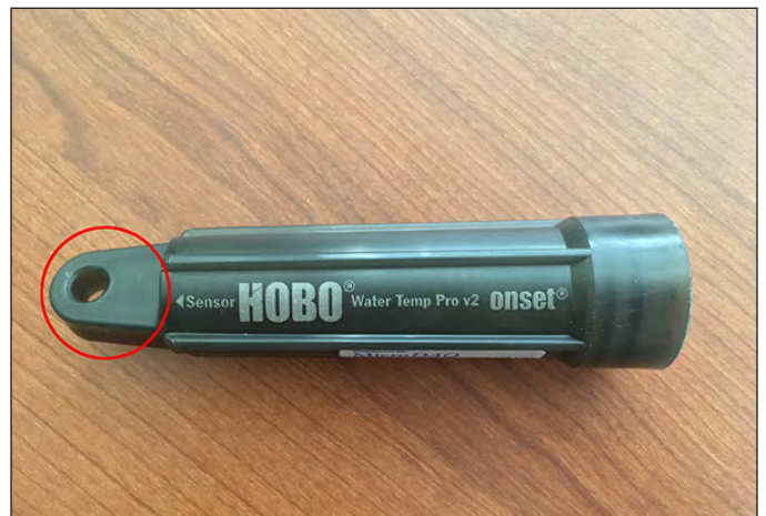
Figure 3.10. Photograph showing Onset U22 data logger with the sensor end highlighted by a red circle.
