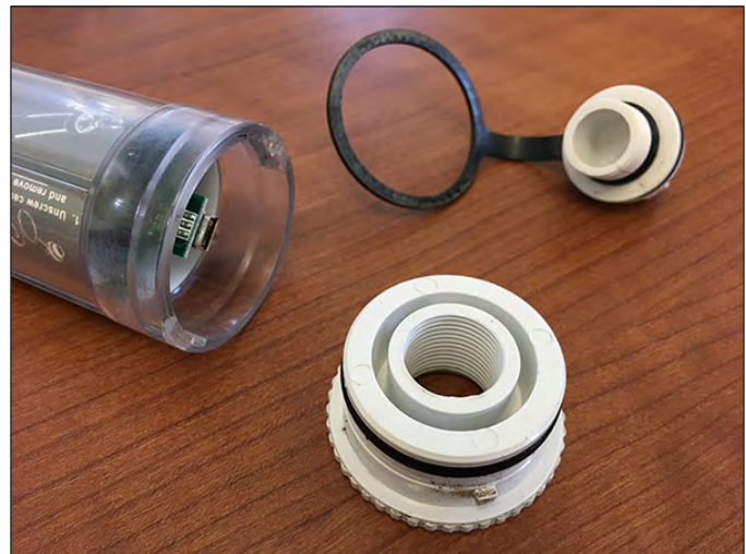
Figure 4.5. Photograph showing Onset HOBOWare Waterproof Shuttle with large cap removed.
