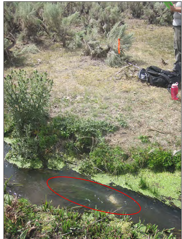
Figure 3.4. Photograph showing data logger attached to a DUCKBILL anchor. Note the thin grey cable to the left of the white PVC solar shield. The actual DUCKBILL is buried in the sediment where the cable disappears and is highlighted by a red oval. Photograph by Brianna Sempert, U.S. Geological Survey.
