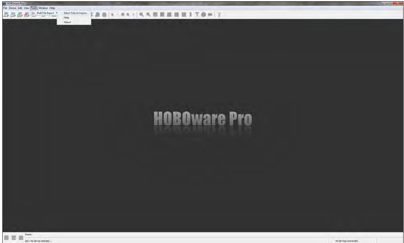
Figure 5.10. Screen capture showing HOBOWare Pro Select Files to Export... option under the Bulk File Export option, under the Tools menu.
