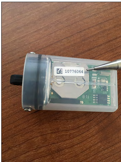
Figure 3.9. Photograph showing serial number placement on an Onset Pendant data logger.
