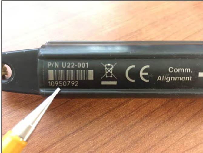
Figure 3.8. Photograph showing serial number placement on an Onset U22 data logger.
