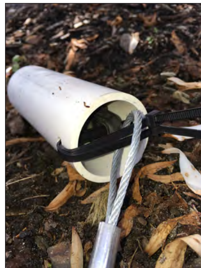
Figure 3.7. Photograph showing Onset U22 data logger inside a PVC solar shield and attached to a DUCKBILL anchor cable with two 11-inch cable/zip ties.
