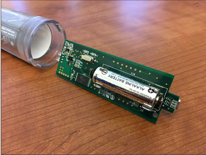
Figure 4.6. Photograph showing Onset HOB0 Waterproof Shuttle with circuit board removed.
