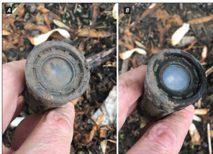
Figure 4.10. Photographs showing Onset U22 data logger with (A) a dirty and (B) a clean optic communications window.
