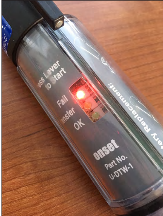
Figure 4.13. Photograph showing Onset HOBOWaterproof Shuttle with a lit red Fail light. A flashing Fail light indicates that data transfer process from data logger to shuttle has failed.
