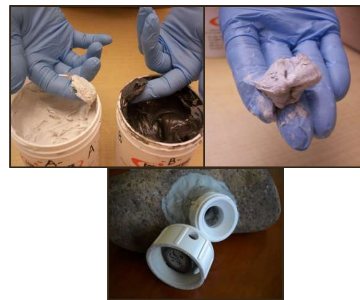
Figure 4. A two-part epoxy is mixed and used to cement PVC containers with temperature sensors to large rocks and cement structures in streams and rivers. A removable screw-top provides easy access to the sensor for data retrieval.
