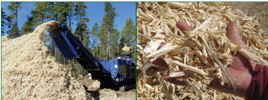
Wood being fed into a horizontal grinder to produce wood shreds (left). Wood shreds that are 2 to 8 inches long and less than 1 inch in diameter are best suited to be aerially applied for hillslope stabilization (right).
