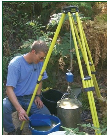
Measuring sediment using a survey tripod.
