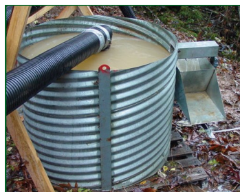
A tipping bucket system and flow splitter are used to measure flow and fine sediment.
