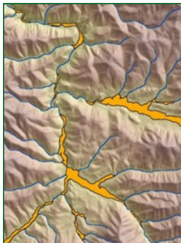
Example VCA output, where unconfined valleys are delineated (orange polygons) and all other valleys outside of the polygon and along stream channels are considered confined.
