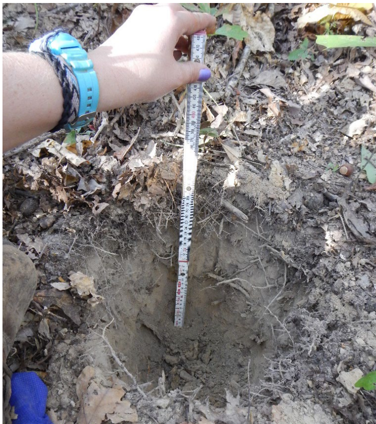
Photo 6. Measuring soil depth to collect soil samples.
