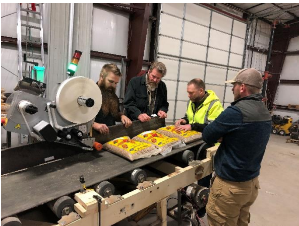
Matt Allen of Mont Taylor Manufacturing inspecting a potential new automated label machine for wood pellets.
