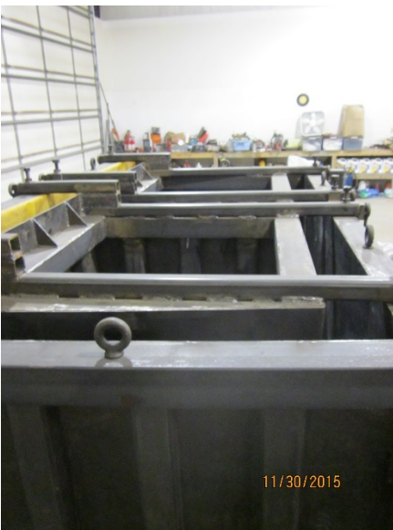
Forms custom built and blocks cast throughout winter months
