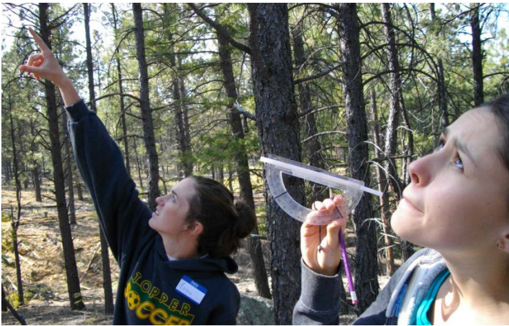
Figure 2 – Picture of students measure trees in the VCNP using instruments they made from protractors and straws.
