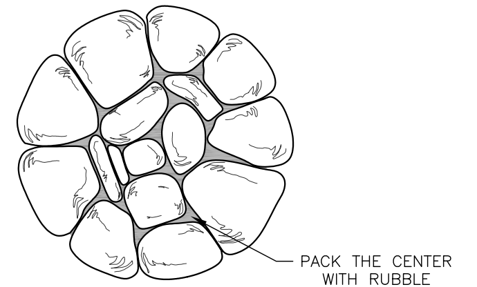
TOP VIEW FIRST LAYER OF ROCK CAIRN OR TYPICAL SECTION OF SHEEPHERDERS CAIRN
