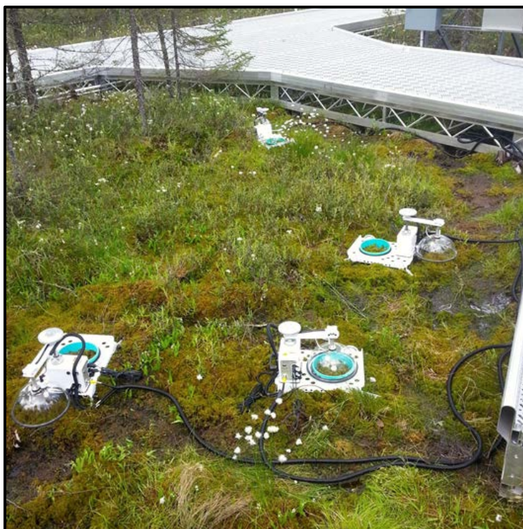
Figure 1. LICOR 8100 clear top soil respiration chambers as installed in S1 Bog to measure Sphagnum NEE.
