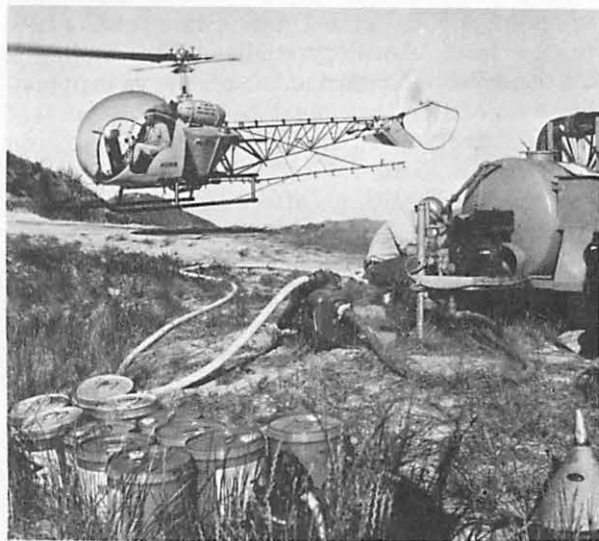
Figure 25.—Safety at all stages of a spray operation must be stressed. Here a crewman responsible for loading the helicopter ducks out of the way while the helicopter lands.
