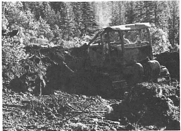
Figure 15.—A pit about 6 feet deep can be excavated on suitable sites, slash pushed into it, compressed, and covered at costs less than those for chipping but more than for tractor clearing and pile burning.
