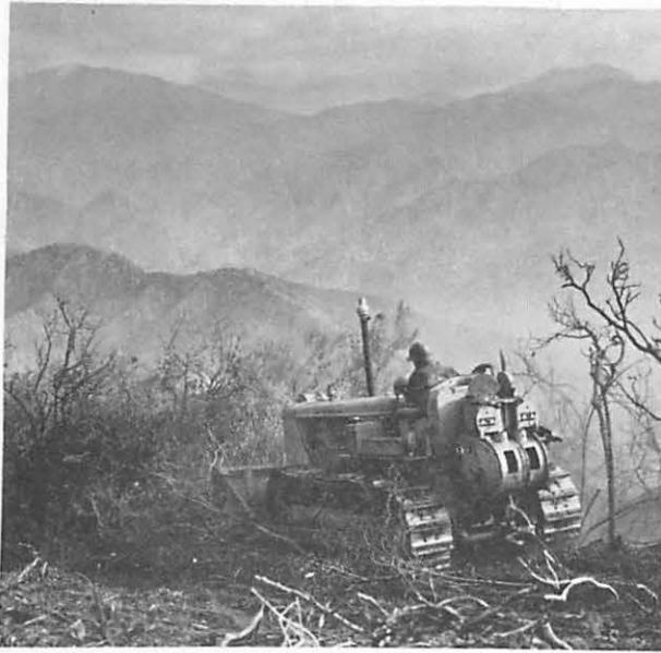
Figure 12.—The bulldozer is more widely used for clearing brush than any other equipment. Soil disturbance can be excessive, however, if the work is not done carefully.
