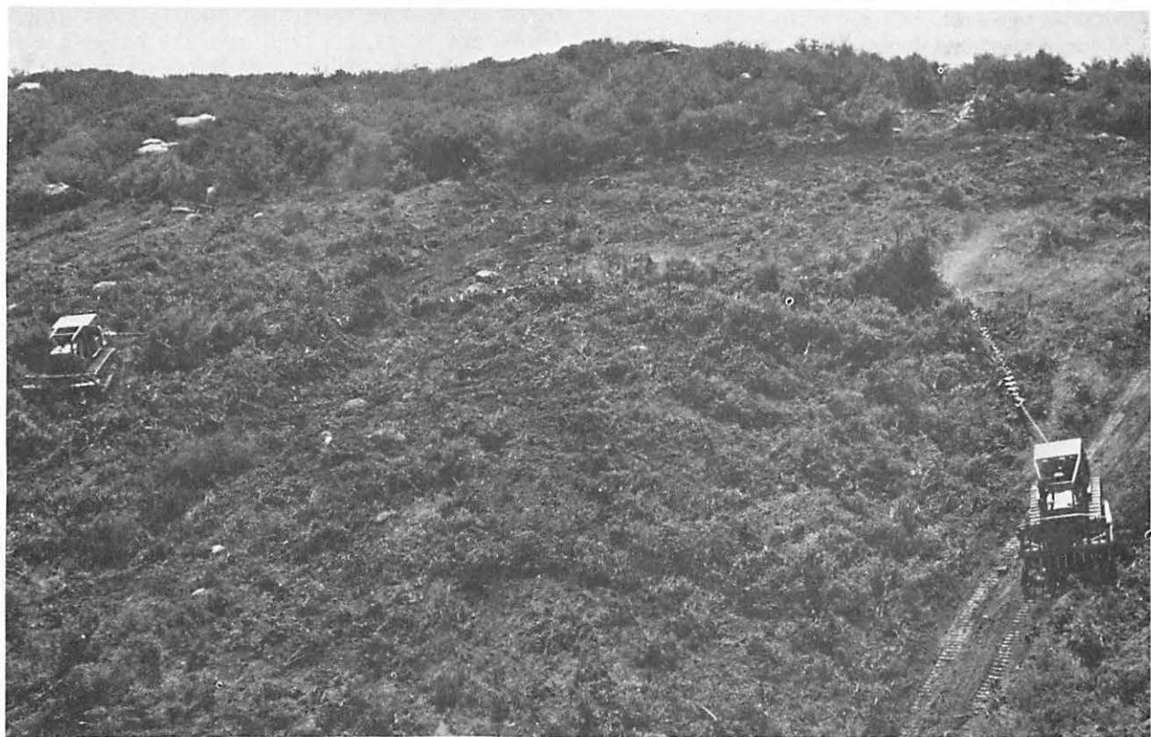
Figure 18.—Two tractors (top), connected by an anchor chain, prepare to crush dense chaparral in preparation for burning, and (bottom) make a second pass in the opposite direction to uproot as much as possible.
