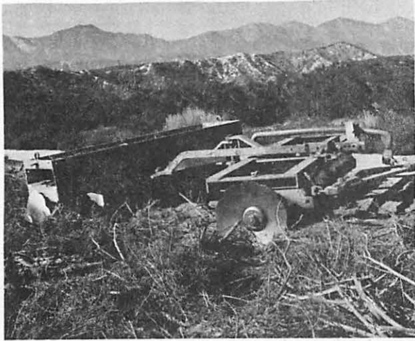
Figure 13.—The heavy brushland disk (left) is effective for light to medium brush, particularly chamise, frequently leaving the site suitable for drilling with the rangeland drill. Heavy chamise chaparral (right) is inadequately prepared for drilling after one pass; a second pass will uproot and mulch more of the brush.
