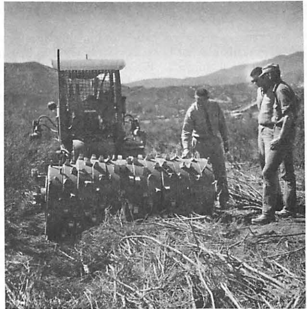
Figure 19.—Various crushers and rollers have been used with the tractor. This 6-foot-wide experimental roller proved helpful for crushing mature brush inside the tractor treads and for forcing broadcast seed into the ground.
