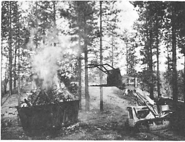
Figure 14.—In one slash-disposal operation, green or dry slash was burned in a portable slash burner as fast as a small tractor-loader could feed slash piles into it.
