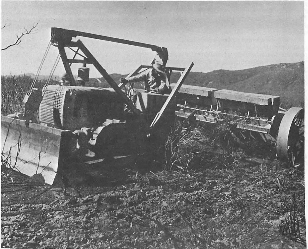
Figure 39.—The rangeland drill is the only large drill rugged enough for use on wildland sites, and it can be damaged. A dozer blade carried just above the soil surface is some insurance against damage.
