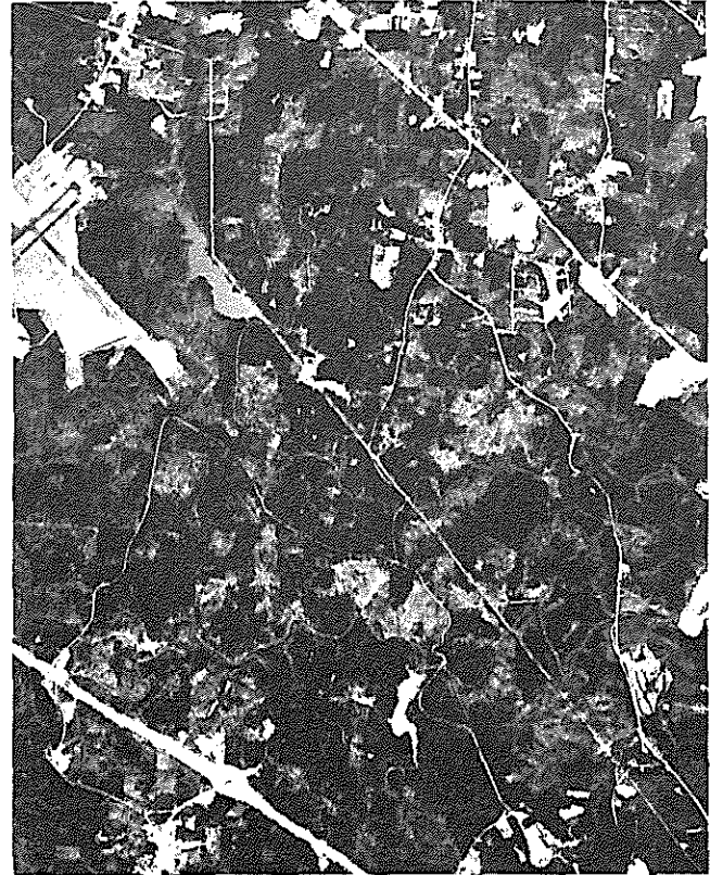
Figure 2—Print of a small-scale (1:78,000), high-altitude, black-and-white photo used as a base map to establish geometrical control of photo-detected tree mortality.
