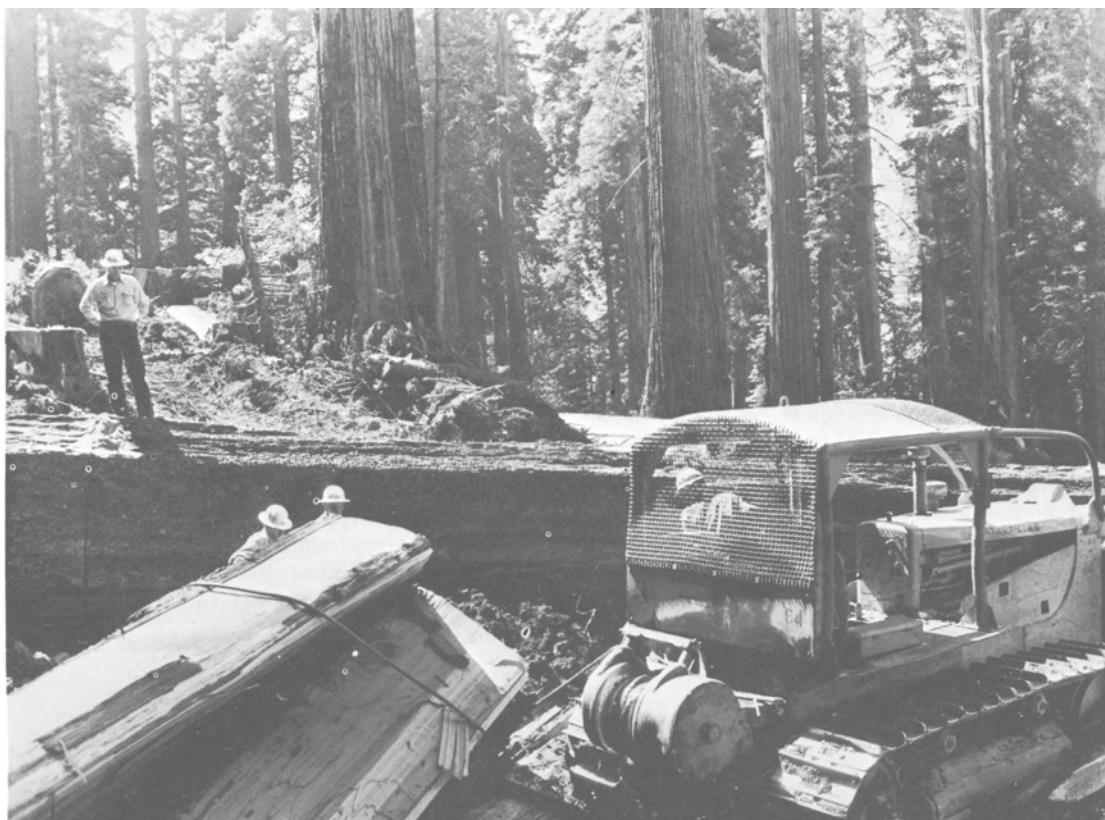
Figure 5.—Skidding production may be estimated rather accurately by the average volume per log.
