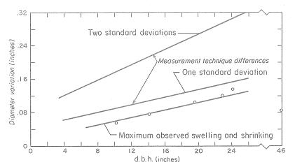
Figure 2-Magnitude of d.b.h. variation of robusta eucalyptus trees due to swelling and shrinking of the bark compared to differences in d.b.h. measurements resulting from individual techniques of using a diameter tape.
