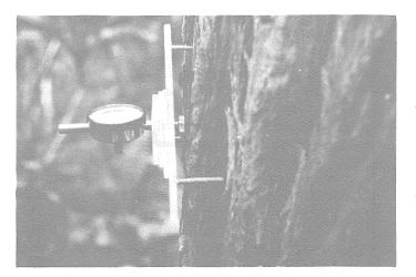
Figure 1–A dial-gage dendrometer to measure diameter change was positioned by three nails driven into the robusta tree. The one-halfinch square of plexiglass mounted on the foot of the spindle minimized abrasion of the bark during placement and removal.
