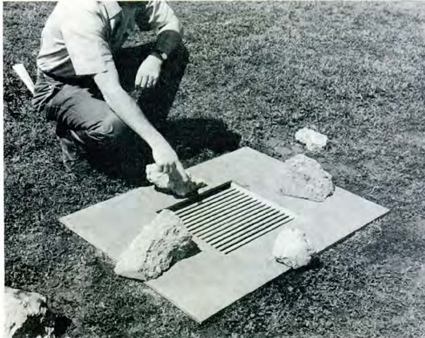
Figure 1.--One of three assemblies of 1/2-inch pine dowels located in the target area. Rubble kept the plywood cover from sliding during the drop impact.
