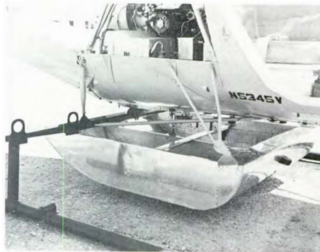
Figure 5.--Filling the Irvin Air Chute tank as it is hovering—or why fire safety officers get grey.
