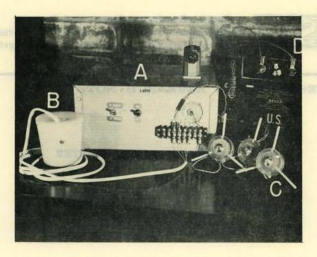
Figure 1.--The fuel temperature counter consists of <u>A</u> a counter-timer, <u>B</u> a pulse generator, <u>C</u> sensors, and <u>D</u> a 24-volt battery.
