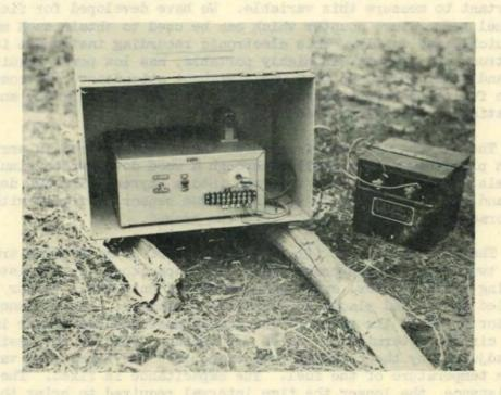
Figure 2.--The fuel temperature counter installed in the field. The pulse generator is buried 3 feet to keep the temperature constant. The counter-timer is protected by the metal carrying case.
