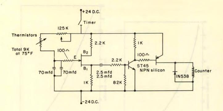
Figure 3. -- Schematic diagram of pulse generator-amplifier.
