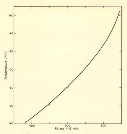
Figure 6.--Relationship between temperature of sensors and pulses per unit of time.
