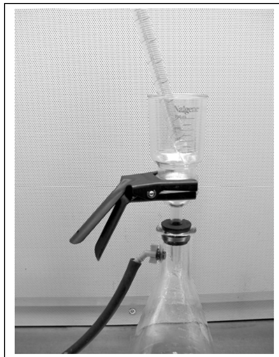
Figure 2—A 100 ml sub-sample of stream water was transferred by pipette and then pulled through a membrane filter with the aid of a vacuum.
