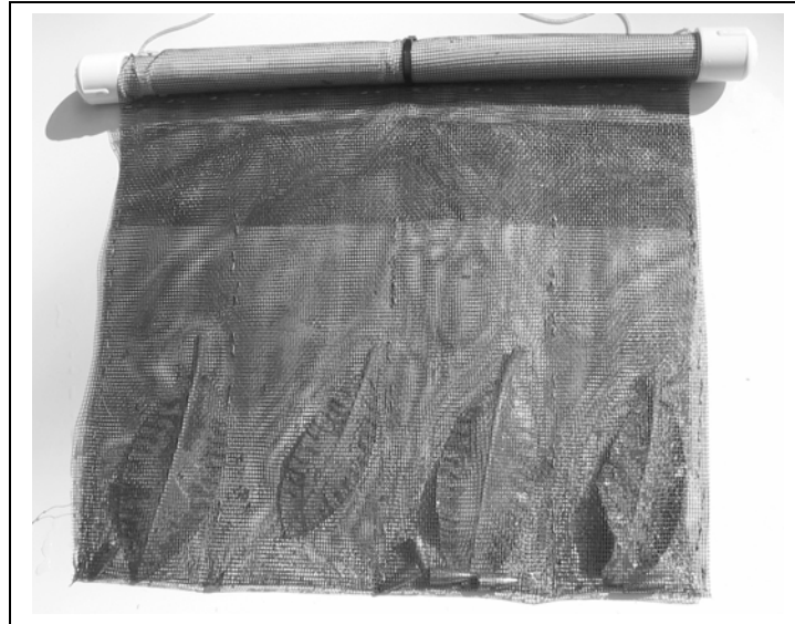
Figure 1—Nylon mesh bag used to float wounded or non-wounded rhododendron leaves in forest streams. The PVC tube provides support and buoyancy.
