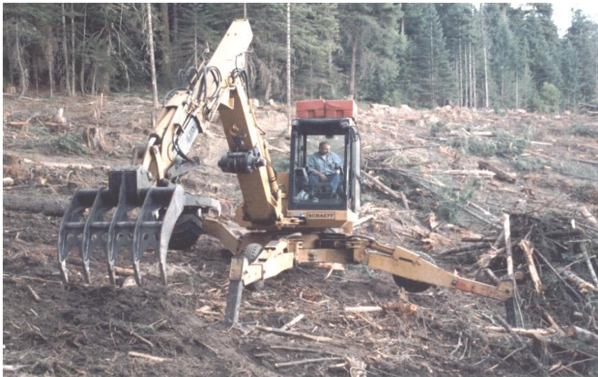
Figure 3 —Spyder is used to prepare sites for planting.
