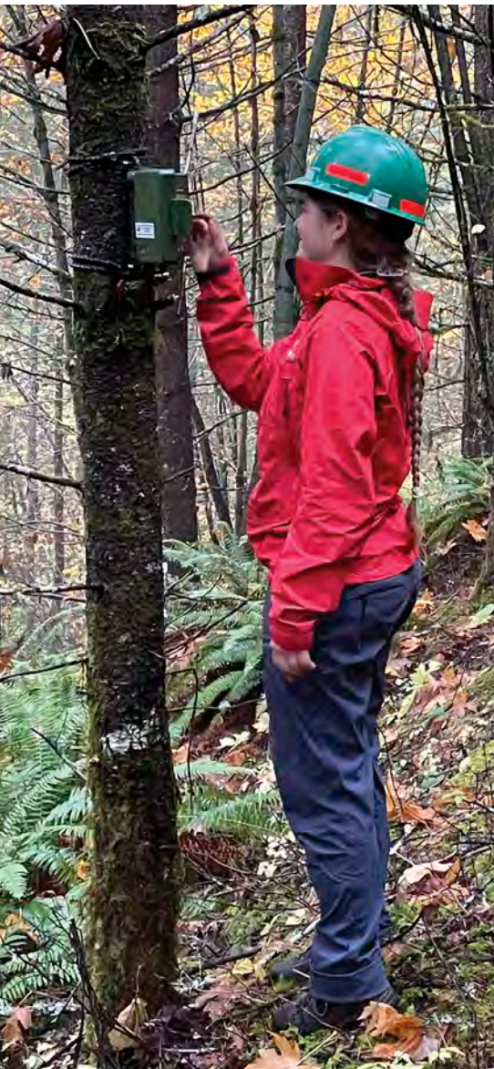
A researcher checks an autonomous recording unit placed to record owl calls. Photo by Jim Swingle, USDA Forest Service.
