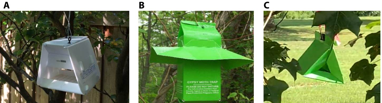
Figure 26. — Lymantria dispar pheromone-baited traps: (A) Moth TrapMonitor (photograph courtesy of Charles Oppenheimer), (B) USDA milk carton trap, (C) delta trap.
