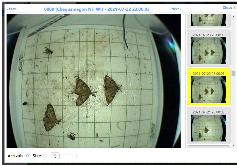
Figure 27. — Lymantria dispar trap catches in pheromone-baited Plurasense Moth TrapMonitor displayed on the web portal.
