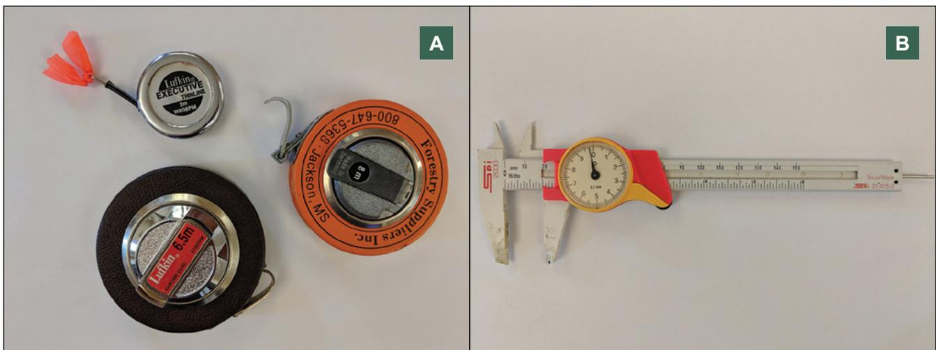
**Figure 10.**—Equipment for measuring trunk diameter: (A) d-tapes; (B) caliper tool. Photos by N.S. van Doorn, USDA Forest Service.
