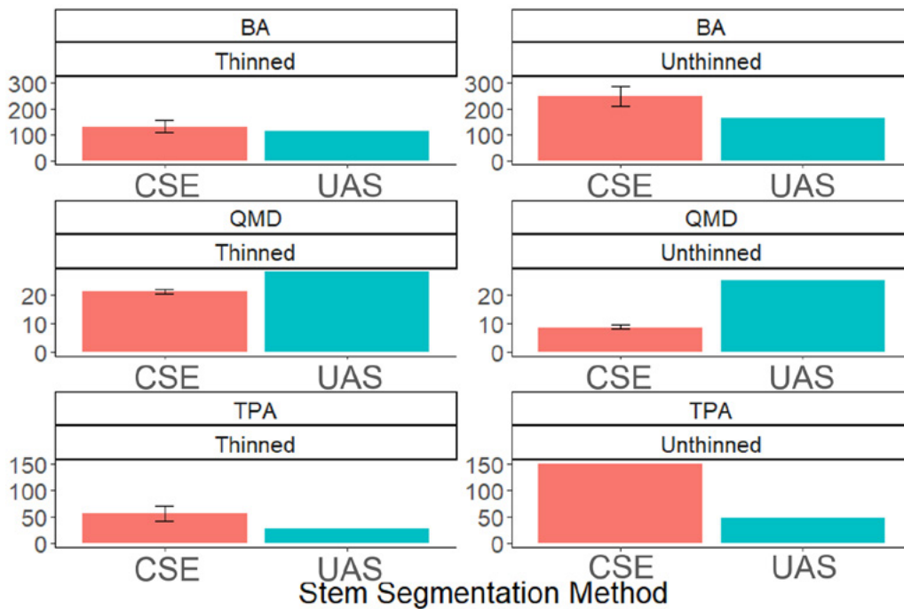
Figure 3.—Common stand exam (CSE) and unmanned aircraft system (UAS) estimates of stand structure in the thinned and unthinned stands as characterized by basal area in units of ft 2 per acre (BA), quadratic mean diameter in inches (QMD), and tree density (trees per acre or TPA). CSE estimates are plot means with 95 percent confidence intervals shown with error bars. UAS estimates do not have confidence intervals since observations were not derived from samples and characterization of UAS estimate uncertainty was beyond the scope of this pilot project.
