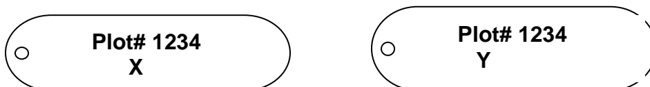
Figure 1.2 – Example of a racetrack tag scribed with Plot ID and witness tree information.
