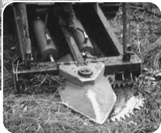
A circular saw mounted on the Bobcat results in a highly maneuverable and efficient tool for removing selected trees in the windbreak renovation project.
