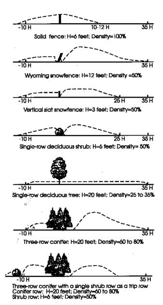
Height (H) equals the height of the snowfence or windbreak. Both height and density affect the amount of snow stored and the area in which it is deposited. Return to the diagram example to compare actual differences in snow storage.
