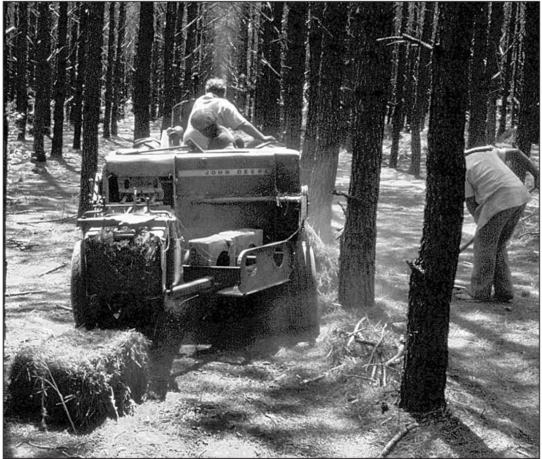
Tractor-powered balers can be used with one person pitch-forking the straw into the baler, another tying the wire or twine around the bale and a third person stacking the bales. A three-person crew can produce 250 to 300 bales per day. Photo: David Moorhead
