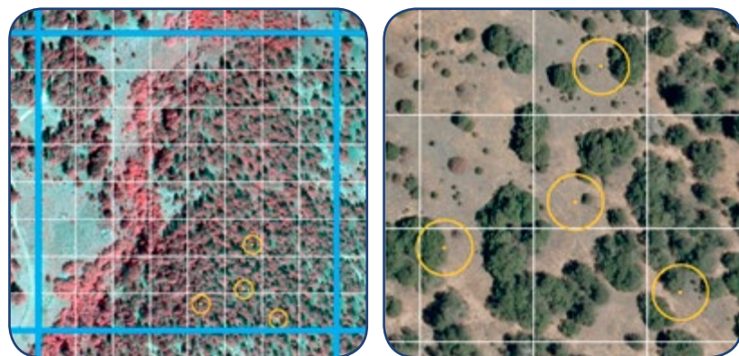
A perturbed FIA subplot cluster (set of 4 circles) is super-imposed upon a high resolution image with a 240-meter grid (blue square) [Left] and 30-meter grid [Right] to illustrate the spatial relationships among the ground data, the predictor layer ground resolution [30m], and the Mapped Atlas product [240m].
