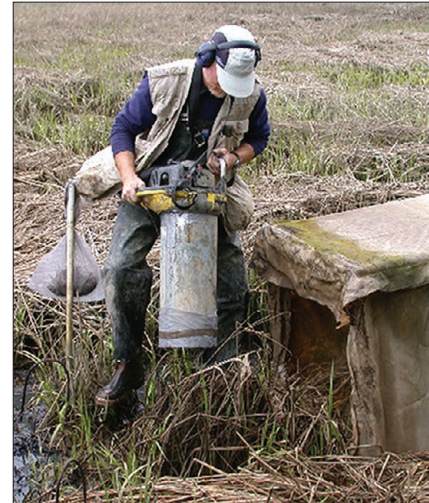
Figure 4-6. Vacuum for collecting insects, using a large-diameter tube (Credit: Fritz Grevstad, Oregon State University)
