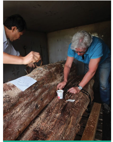
Establishing best temperatures to kill rapid ‘ōhi‘a fungus on logs by installing thermocouples as part of steam/vacuum treatment. Photo by J.B. Friday, University of Hawaii.
