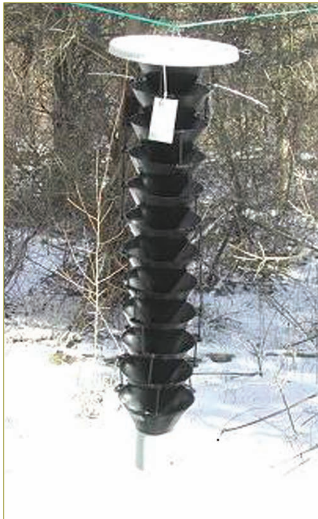
Figure 1.—Lindgren funnel trap. Photo by Pennsylvania Department of Conservation and Natural Resources.
