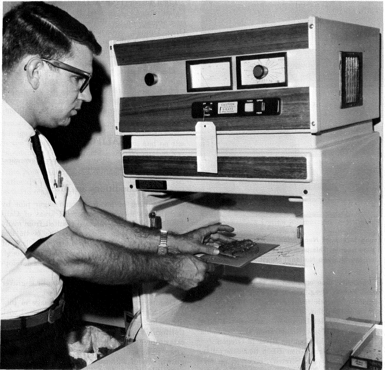
X-ray pictures of ponderosa pine bark samples help determine population trends of the western pine beetle. Beetles hidden beneath the bark are counted on the X-ray. (San Francisco, Calif.)
