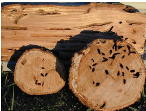
Figure 1. Structural damage and degrade in lumber quality caused by red oak borer larval feeding. Photo by F.M. Stephen, Forest Entomology Lab, University of Arkansas, Fayetteville, AR.
