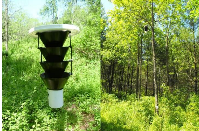
Figure 17. (Left) Four funnel Lindgren trap baited with a walnut twig beetle lure. (Right) Baited funnel trap hangs in a declining walnut tree canopy.
