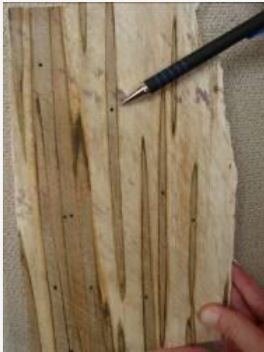
Figure 12. Characteristic staining of wood caused by Columbian timber beetles. Photo by Linda Williams
