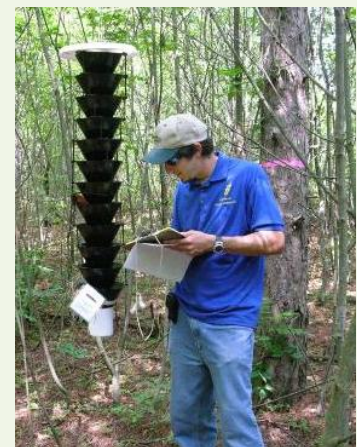
Figure 14b. Lindgren funnel trap used for European woodwasp detection (M Guthmiller).
